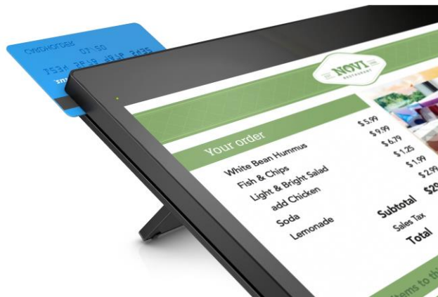
MSR is behind the top section of the display (badge authentication only*)
